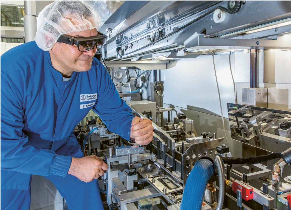
During maintenance procedures, production engineers can establish a live connection to remote technicians via augmented reality goggles.
