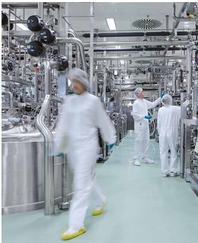
Biopharmaceuticals are cultivated in bioreactors with a capacity of up to 15,000 litres.
