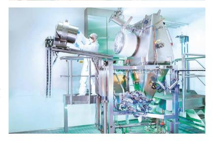
Active pharmaceutical ingredient plant: above: Transition through the personnel air lock to the closed filling area. below: Feeding an active ingredient into a micronization unit.
